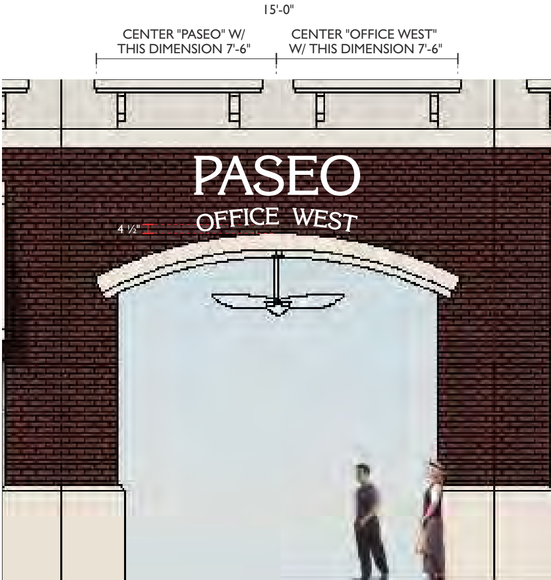
BUILDING "K" EAST ELEVATION DETAIL 1/4" = 1'
