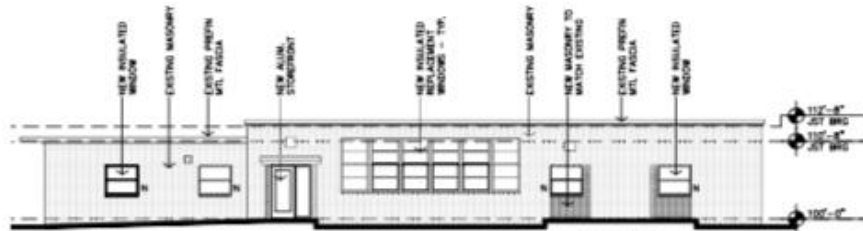
C BUILDING B EAST ELEVATION 1/4"=1'-0"
